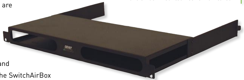
This SwitchAirBox version delivers cooled air from the front of the cabinets to the side fans of rack mounted network switches.
