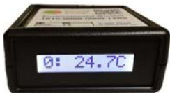
Environmental Monitors for humidity, temperature and differential pressure data
