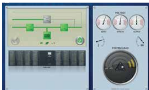
System status, measurements and single-line diagram.
