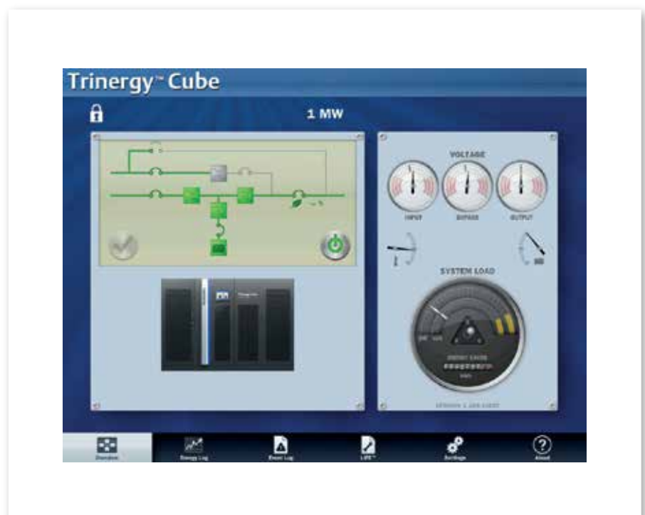
Trinergy Cube LCD touch screen: interface for data tracking, logging and event analysis
